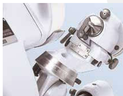
Radial positioning using a setting finger
